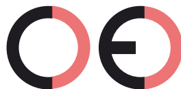
False CE Mark (too far)
