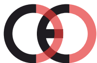
False CE Mark (too close)
